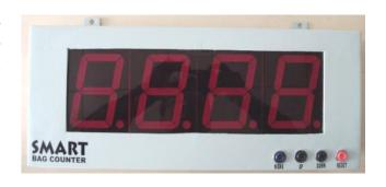
The instrument has single chip microcontroller, smps based power supply unit, switches for counters(UP,DOWN, MENU & RESET SWITCHES), large seven segment display unit for showing counts, precise counting, high speed, durability and is applicable for reminding the quantity for loading the vehicle. By using DUAL OPTICAL BASED SENSORES instead of conventional SINGLE sensors gives better, precise & prompt readings with metallic body enclosure for longer life in dusty and rough industrial atmosphere.
